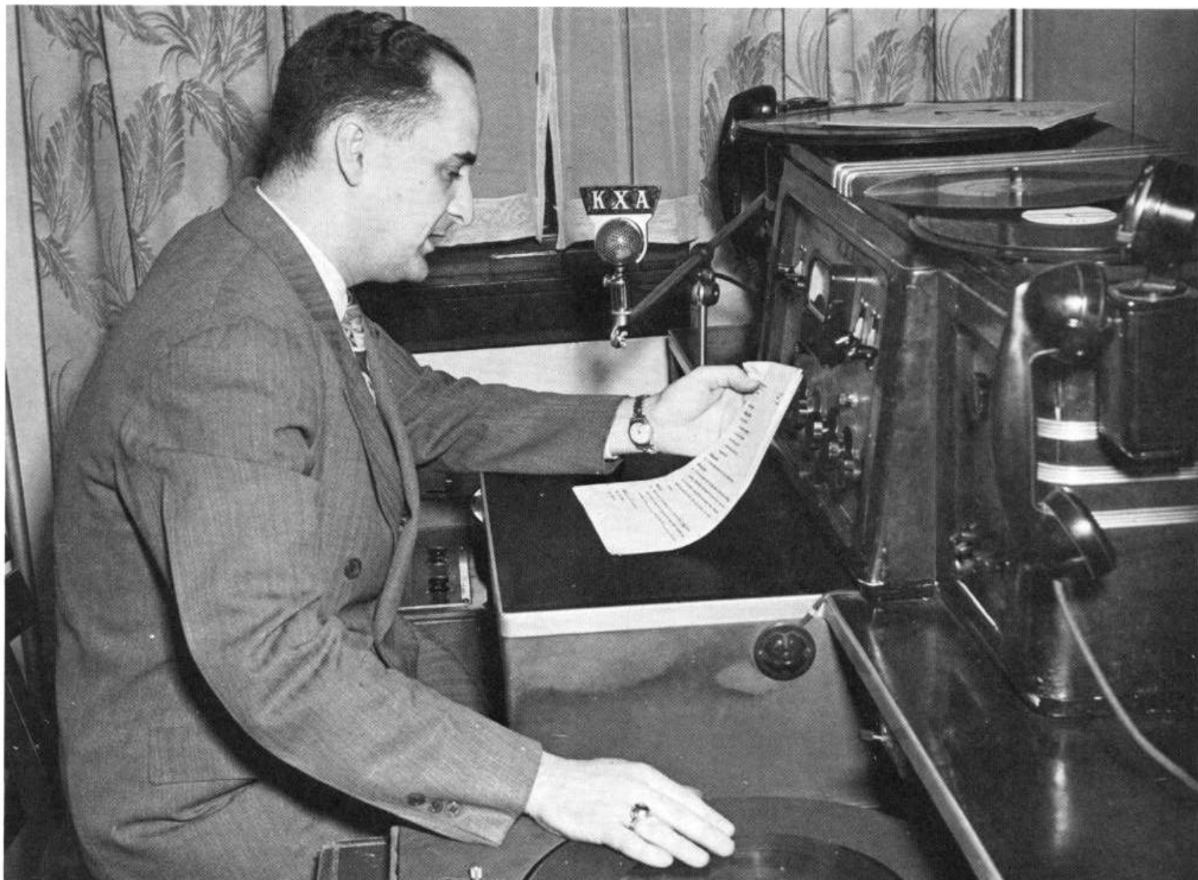
John H. Dubuque , chief engineer and popular announcer at KXA , Seattle in 1947. He's shown here at the control board of KXA's Bigelow Building studio, reading a "spot" announcement and preparing simultaneously to cue up a sound effect record on the near turntable.
