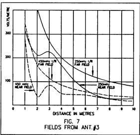
This can also affect the relationship between the electric and magnetic field components and cause the apparent free space impedance anomalies mentioned above. At 250 mHz the far field measurement error at distances between seven and ten metres from a source two metres in length is between -9 and -11 dB. At 450 mHz the error two metres from the same source is -13 dB and about -5.5 dB at distances of 9 to 10 metres.
